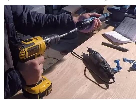
And file the freeze plug baffles...
