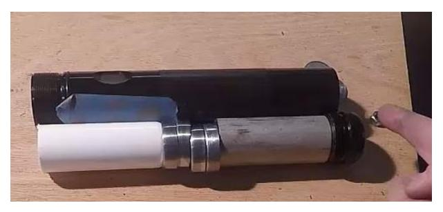
The barrel screws on the right, and the bullets come out the left... This is simple. If you wanted, you could add spacers between the baffles, or cut down some of the PVC, and add more baffles, etc. But this was quick and dirty.
