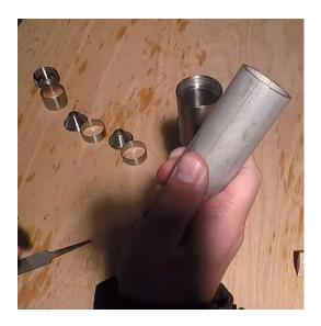
One thing that helped, when putting them in there, was to use another similar sized piece of tube that fit in the inside of the silencer – to be able to "ram down" the baffles because it helped put equal pressure around the sides of the baffle to keep it from getting pushed to far down on one side and stuck:
