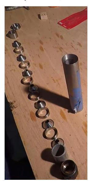
Then, you probably want to start with the muzzle end of the silencer and the blast chamber and work from there... remember to start with the stainless-steel blast chamber and baffles if you are using titanium on the rest:
