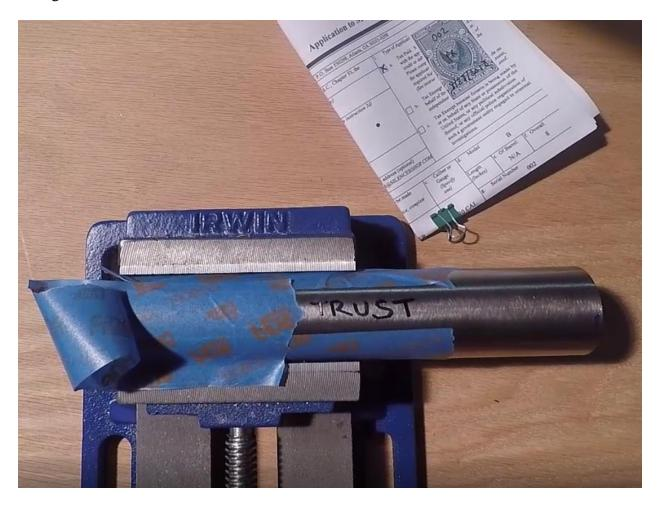
As you can see, I used some painter's tape to put down to guide me. I also simply used a permanent market to write on the metal of the tube the words to guide my engraving. Simply engrave until you reach the proper depth, pretty self-explanatory here:
