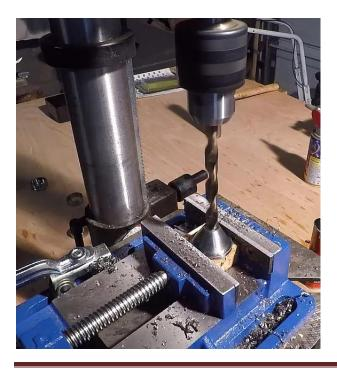
The other thing that I'd like to point out, is that in the video step-by-step you see that I tried taping all the baffles together, one on top of another and just drilling straight through... that turned out not to work too great.
