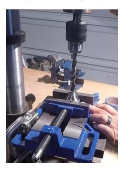
This is pretty self-explanatory, drilling holes... but one thing that might help, that you can see in a closeup here is that I put a wooden block underneath the baffles, to help hold it in the vice:
