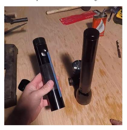
When you do that, you basically just screw off the end pieces – one side has the bulbs and the other has the battery compartment, easy peasy.
