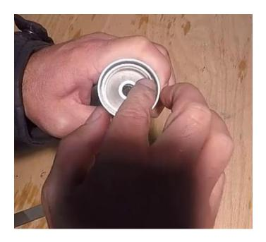
For me, I got to the end, and when I went to screw on the end cap - it wouldn't screw down all the way with the last spacer sticking up after the last baffle. This is good, because it meant I could file down the last spacer until it was just the right height and the fit was nice and tight and the end cap screwed on fine:
