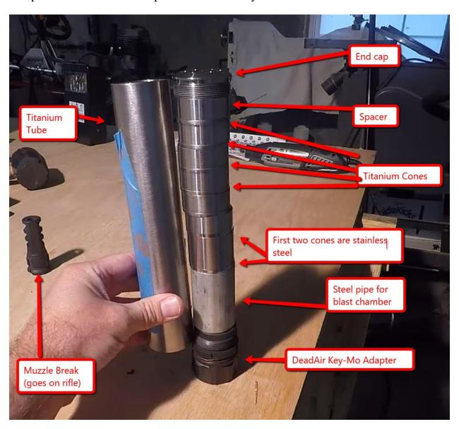
The cone baffles and spacers are machined so that you put the cone on, and then the spacer sits right on top of it:
