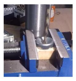
I believe these are made out of aluminum which makes them a lot easier to drill. Drill through the one side, then turn over and deburr the ragged edge on the other side using the drill
