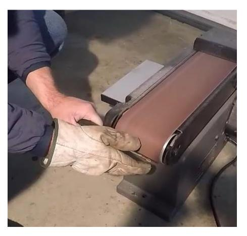
Once you drill the center out of the baffle, you can stick a screw driver through it, to hold it, and using a glove, let it get the high-speed sanding on the belt sander...
