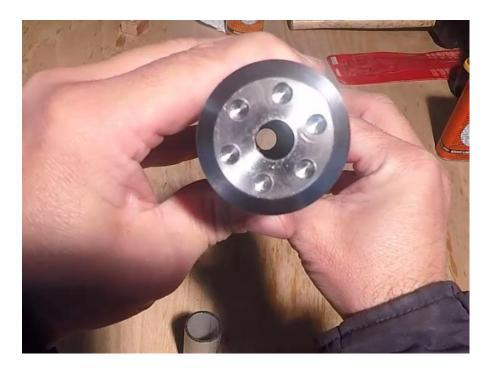
I did not use one, but there are things called "bore rods" that might help you to make sure that your alignment is correct and you did well enough on the holes. If you use that and find that it's not aligned correctly, then you could go back and re-drill the problem baffle.
