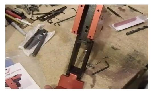
Then using your router, and the included depth gauge – using the (A) slot – start milling at the first hashmark ...
