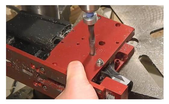
Then using the 5/32" drill bit, drill the trigger hole ...
