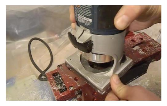
When you complete this step, the entire fire control pocket, along with the rear shelf will be milled and looking nice as in the picture below!
