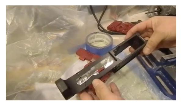
And your safety selector and trigger and hammer holes all drilled out:
