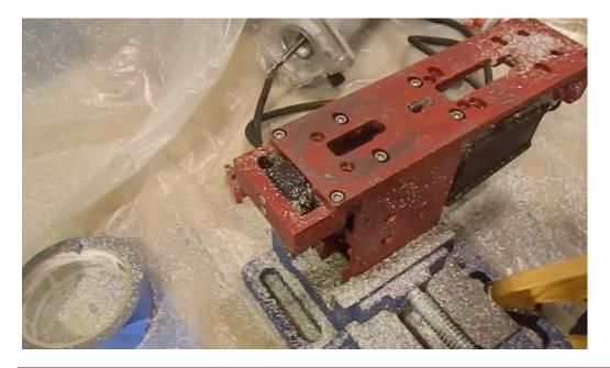
When you complete this step, you will see that the rear shelf is completely milled out and that the trigger slot and the rear shelf are now done!
