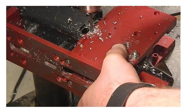
Then flip the jig over and repeat ALL three holes on the other side. Make sure that you are drilling the correct holes at the top of the jig template and that they all line up!
