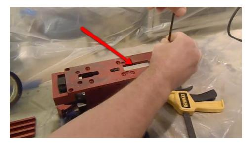
So you'll need to remove the screws and flip it around so that it now sits over the rear shelf/fire control pocket area (the area closest to the buffer tube, or left side of this picture), as shown below:
