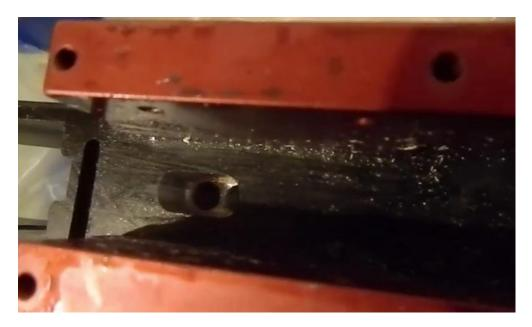
And by the end of the process, you will have drilled and then milled all the way through the receiver giving you a nice trigger hole as shown in the next picture:
