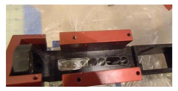
Again, use the (C) slot of the depth gauge, and start with the first hashmark to set your milling bit to in the router, and using the  $1/8^{th}$  inch depth passes, start to mill the drill holes you just drilled in the fire control pocket ...
