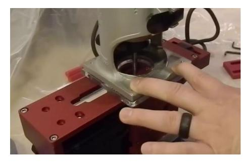
Take your time, and when you remove all that you can at the one hashmark – you simply turn the router off FIRST, then remove from the jig and move to the next  $1/8^{\text{th}}$  inch hashmark and repeat the process. Here's what the milling is accomplishing, see how it removes the material between the two holes that you just drilled:
