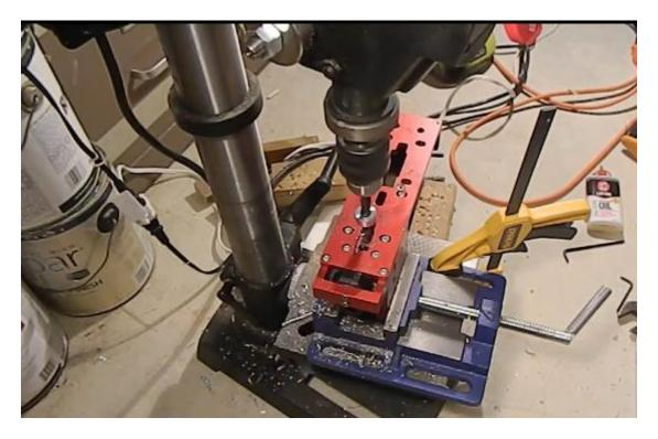
Then you'll remove the drilling template from the jig, and using the depth gauge again set your router end mill bit to the first hashmark of the (B) depth gauge ...
