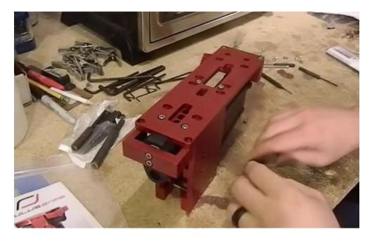
Then you're going to drill those two holes for the trigger slot ...
