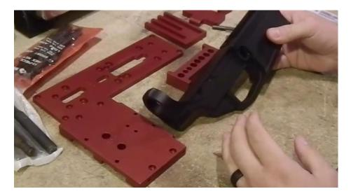
And then you'll put on the front takedown lever, the rear buffer tube support, the side plates and the top plate ... All the parts are attached by Allen Wrench screws, making the entire kit very secure and solid:
