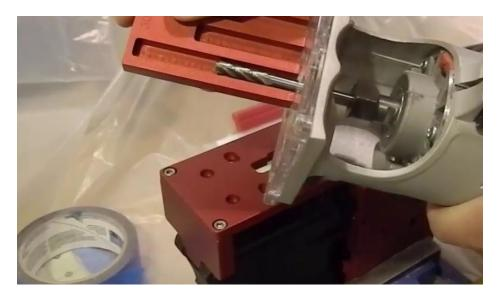
When milling, you start at the first hashmark and drop the mill into one of your drilled holes. Then you slowly go in clockwise circular motions removing bits of aluminum and attempting to eliminate all the material in between the two holes with the mill.
