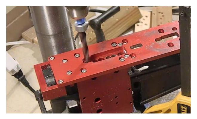
Making sure to stop every once in a while and make sure your drill bit stop did not come loose, so you're drilling to the proper depth – and also use plenty of oil to keep the bit from getting too hot and to help extract as much material as possible:
