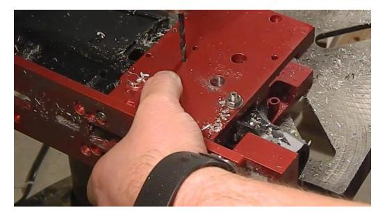
And then the hammer hole using the same size drill bit ...
