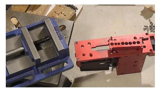
Using the (B) mark on the depth gauge, along with the drill bit stop, will set the proper depth for drilling ...
